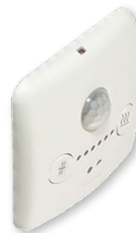
Figure 16. Sensor module for used together with VAV controller for demand-controlled ventilation. Selected as a product accessory and mounted in the face plate or on the wall.
